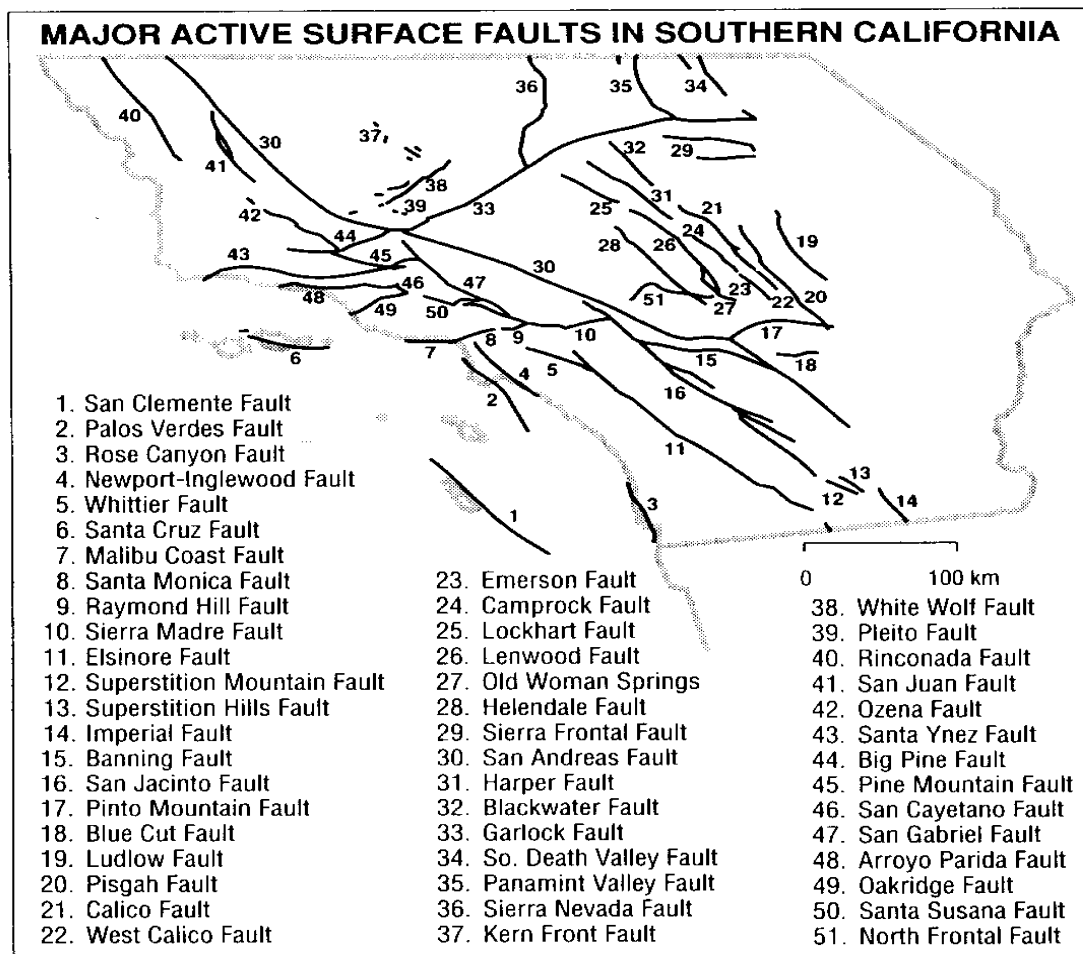
Map 5-2: Major Active Surface faults in Southern California
